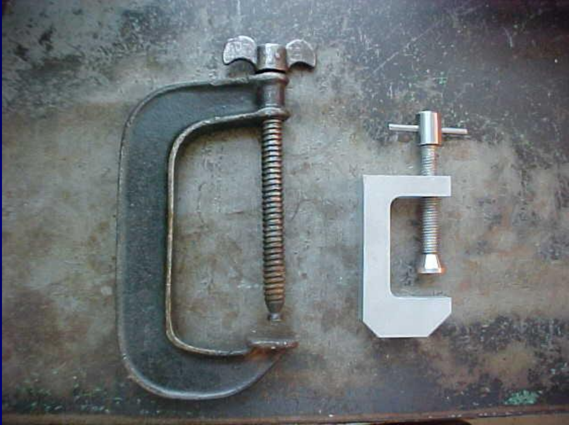
C-clamps formed by casting (left) and machining (right)
